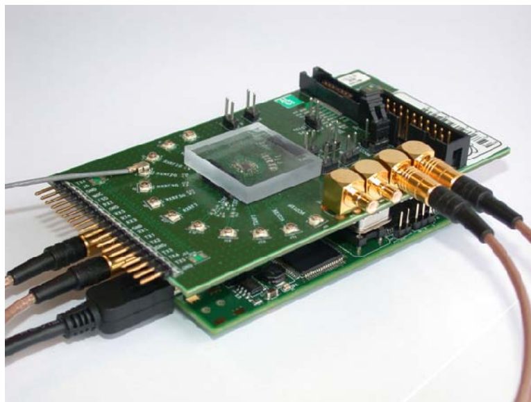
Figure 36: Integrated Sensing Engine: SPIDER PCB coupled to SCALDIO RF module.
